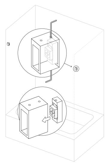
Screw in Shower Rod Bracket on Slider Panel side wall.
