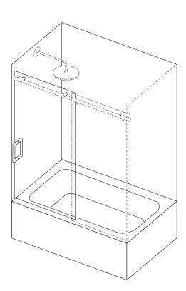
If your shower head is on the left, the Slider Panel should be installed on the left side.
